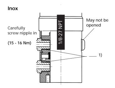
1) Sealing compound standard (e.g. Loctite 326, activator 7649) Sealing compound for sealing material CR (e.g. Leak Lock)
